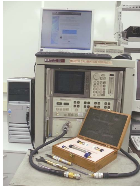
The iPIMMS workstation together with the NPL-traceable artefacts used to error correct and check the system.
